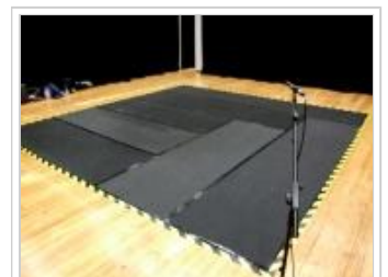
The 5m x 5m capture area is comprised of an array of 4mm thick rubber matting in a square formation that emulates the floor-
