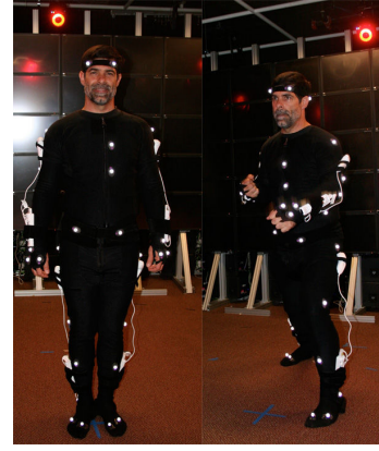
Fig. 2: Data collection: an optical motion capture system and a 3D acceleration sensor based data acquisition system are used in parallel. There are 45 retro-reflective markers and eight sensors (four Wii TM Nintendo controllers) attached to the performer.
